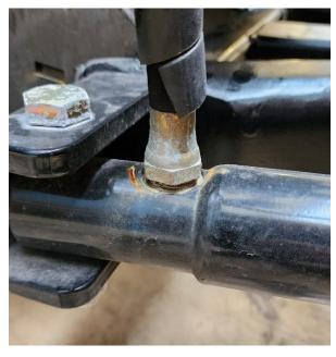
**STEP 3**Disconnect A-frame pin for lift cylinder.
