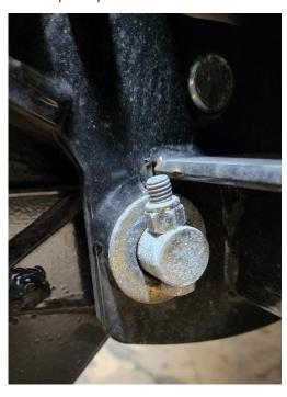
**STEP 11**Reinstall lower mounting pin to secure the lift cylinder to the Arctic Razorback Retrofit Kit A Frame. Reinstall cotter pin.
